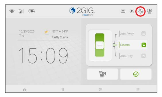
Accessing the **Settings** menu is only available when the system is disarmed. An error message "The operation is not allowed while the system is armed" will appear when users tap the Settings icon in **Arm Away** or **Arm Stay** mode.
