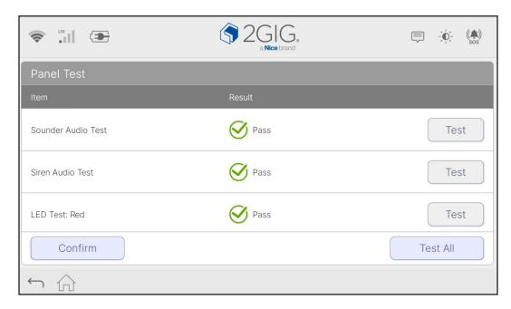
Tap "Test" next to each item to run individual tests, or tap "Test All" to run all tests sequentially. During LED Tests, the Panel will illuminate the corresponding color and prompt the user with a question: "Is the LED displaying Red/Green/Blue/White?" or "Is the LED off?"
