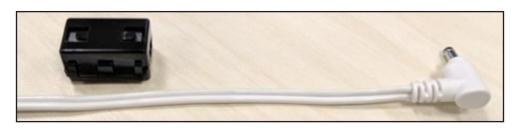
2) Open the clip on the Ferrite Core.
